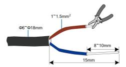
step 3 Insert the stripped DC cable into the port "24V OUT +" and "24V OUT -" of the Logger1000.
