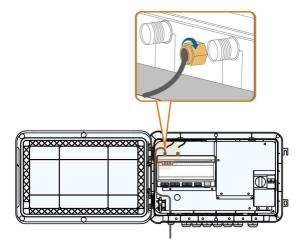
step 5 Place the sucker antenna base on a metal surface outside the container.
