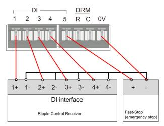
figure 7-3 Wiring of the active power dry contact
