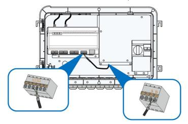
step 8 Pass the external communication cable through the "RS485 – 2/IOM" waterproof terminal at the bottom of COM100 and connect the cable to the AI/DI port on the I/O module.
