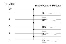
In Germany and some other European countries, the grid company uses the Ripple Control Receiver to convert the grid dispatching signal and send it in a dry contact manner. In this case, the plant needs to receive the grid dispatching signal in the dry contact communication manner.
