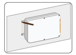
step 3 Drill the holes with a drill according to the marks made before.
