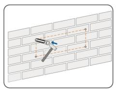
step 5 Use the nuts, flat washers, and spring washers in the delivery accessories to fix COM100 on the installation surface.
