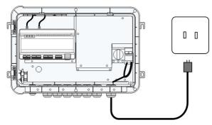
step 3 Strip and connect the cable to the corresponding terminal inside the COM100.
