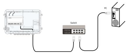
figure 5-2 Connection to PV background system
