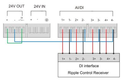
figure 7-2 Wiring of the reactive power dry contact
