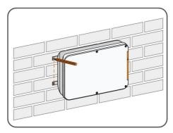
step 3 Drill the holes with a drill according to the marks made before.
