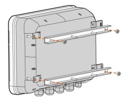
step 2 Fix the mounting-brackets with the clamps by using the nuts.
